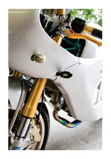
INSTALLATION OF OBERON TURN SIGNALS ON A DUCATI PAUL SMART: YOU CAN MOUNT THE OBERON TURN SIGNALS IN THE "STOCK" LOCATION (BLACK OBERON) OR WHERE THE FRONT FAIRING ATTACHES TO THE FRAME (SILVER OBERON).
